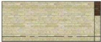
Buff detail brick in caledonian buff blend by ibstock. stretcher bond with bucket-handle pointing in o.b.m.
